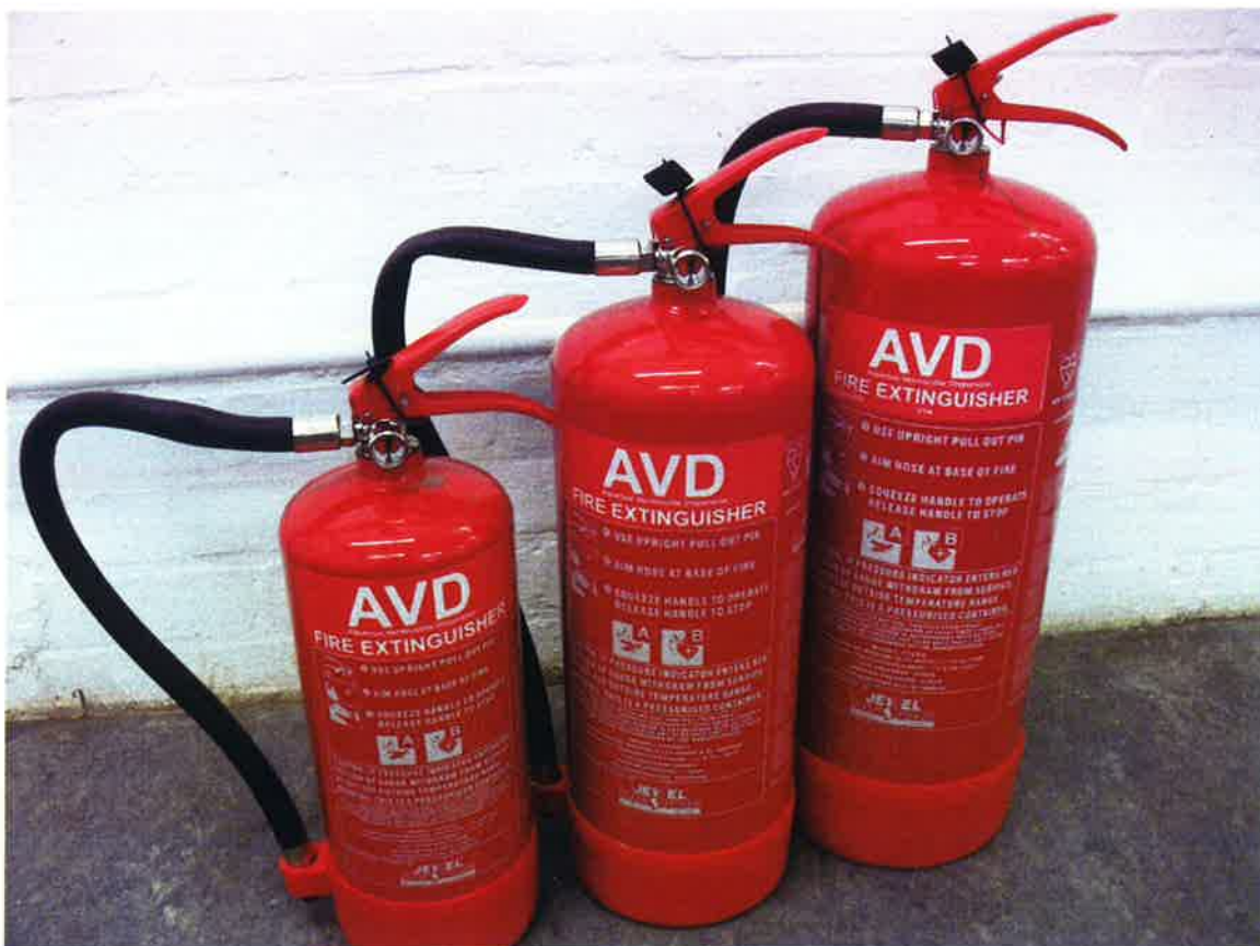
Figure 1 – Jewel Saffire Products Ltd 3 litre, 6 litre and 9 litre Aqueous Vermiculite Dispersion (AVD) fire extinguishers received.
